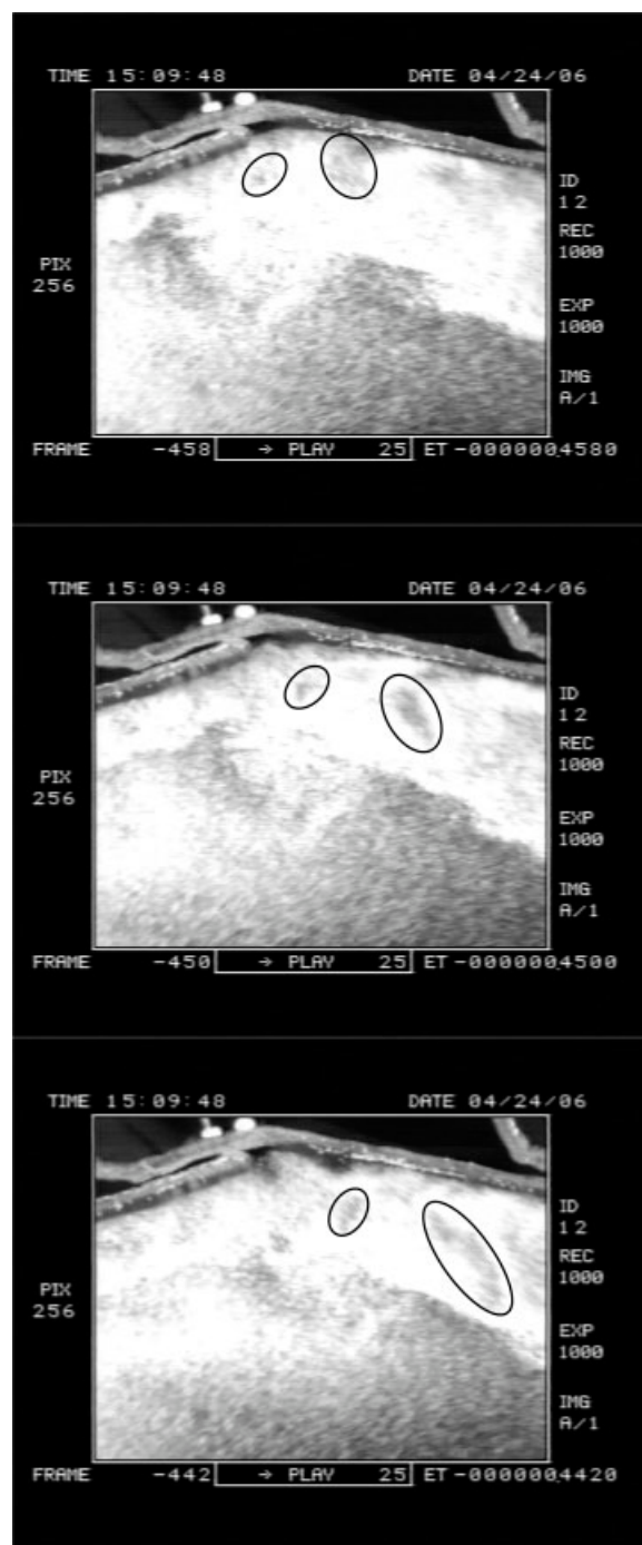
Figure 11. Fast digital camera analysis of the motion of 1G-Geldart B particles near a tangential gas inlet slot of the fluidization chamber.
